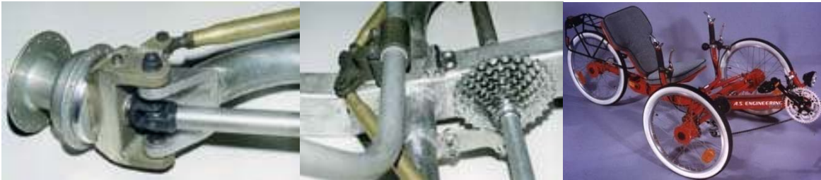
Above are images of the AS Engineering's S327. Details of the fwd system are shown in the left two images.
