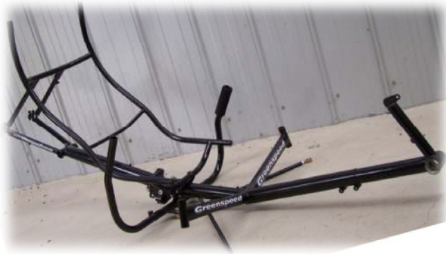
Above: A Greenspeed trike frame assembly complete with steering and bottom bracket shows how the seat is an integral part of the trike frame adding stiffness to the rear end.
