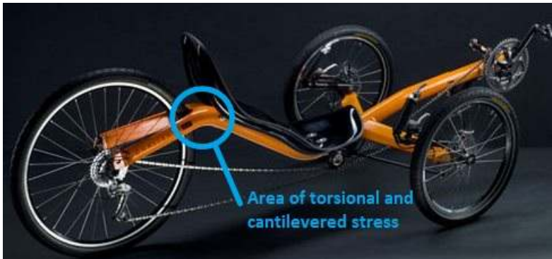
Above is a Challenge Ligfietsen Trike that uses angled dual cantilevered stays. The mark-up shows where the stress is concentrated.
