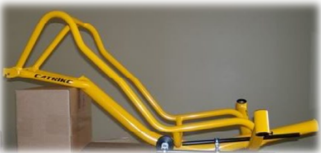
Above is a Catrike frame assembly with chain management attached. This 3-D space frame implementation cleverly doubles the seat frame tubes as the Seat Stays.
