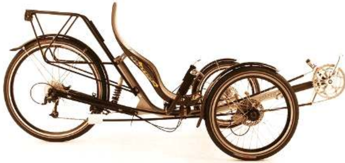
Above is the Optima Rider shown with rear suspension. The larger rear wheel defeats the need for suspension, as it already gives a smoother ride.
